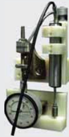
▲ Cylinder Height Data Acquisition System
