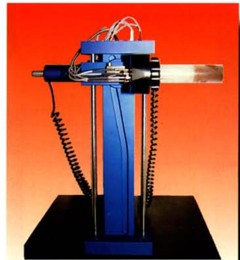
Close-up of Cloud and Pour Point Analyzer Completing a Determination
